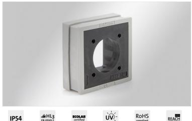
The grommet QT-AT-FL is constructed on the basis of a large QT cable grommet. The polyamide body is moulded with elastomer. All square flanges with dimensions 19.8 x 19.8 mm (M23) can be integrated.
